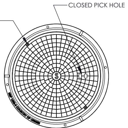
BOLT-DOWN WITH CLOSED PICK HOLE COVER
